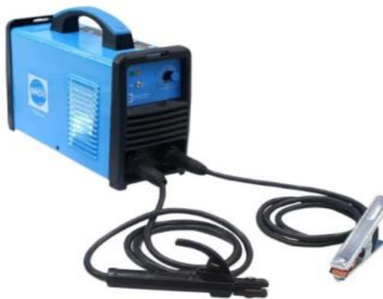
Gambar 1. Las SMAW ( Shielded Metal Arc Welding ) Sumber : dok.2023
