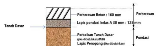
**Gambar 4.** Rencana Lapis Perkerasan Kaku (Rigid Pavement)
