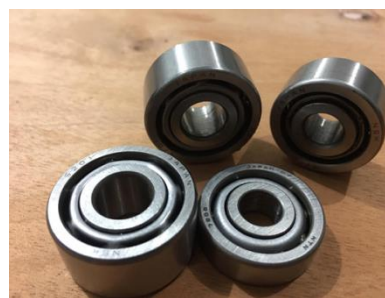
Gambar 1. Bantalan single dan double row angular contact ball bearing
