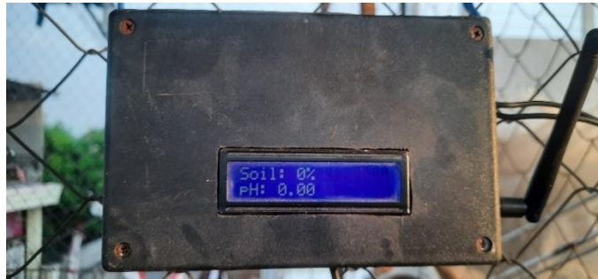
Gambar 39. Panel interface control
